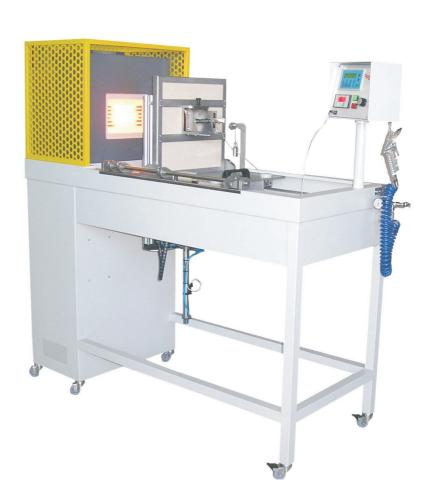
Exposure to a source of radiant heat
